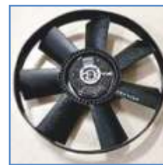
Electronic Viscous Fan for enhanced fuel economy
